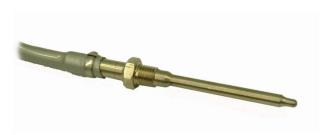
This sensor uses a K type Chromel/Alumel thermocouple and is intended for use in high temperature, high vibration environments. units and data loggers support K type thermocouples. The sensor is short and compact to minimise its susceptibility to vibration.
